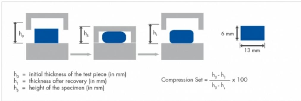
The specimen is compressed by 25%. The compressed specimen is heated to the test temperature. DIN ISO 815 describes two methods.
